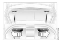
1. Pull the corresponding lever to release – see arrow
